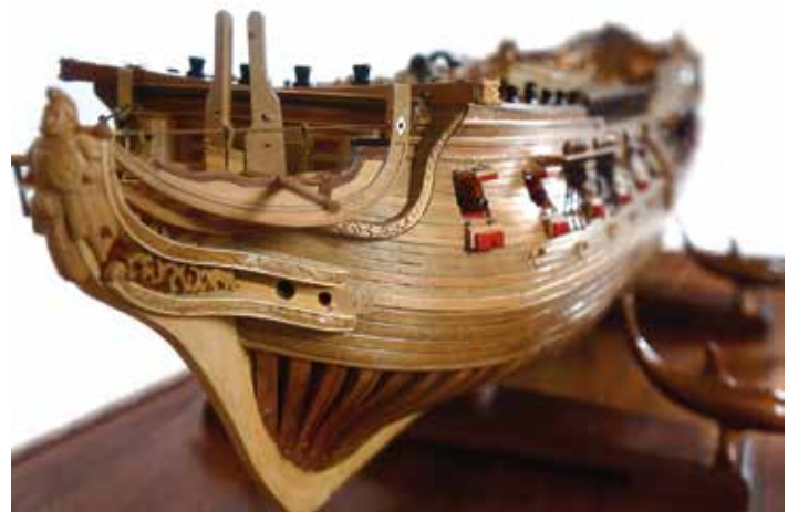
Master modeler Ronald Roberti’s exquisitely detailed model of the USS Confederacy illustrates how eighteenth-century shipwrights documented all the details of a proposed ship’s designs for approval before Computer Aided Design (CAD) or even much skill in drawing flat representations of compound ship hull curves.
