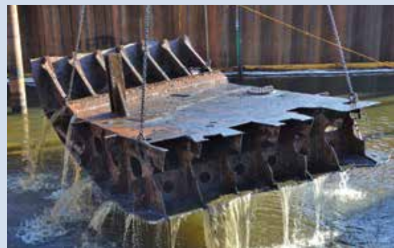
Lifting out a section of Davy Crockett’s double bottom, August 18, 2011.
